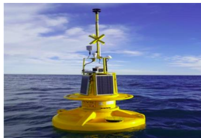
Gambar 13. Alat Deteksi Tsunami ( Tsunami Buoy )
